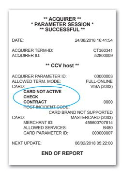
This receipt is printed if the change has not been successful. In this example, the VISA card has not been added correctly or the Merchant ID has not been changed correctly. The message 'CARD NOT ACTIVE, CHECK CONTRACT' is printed on the receipt.
