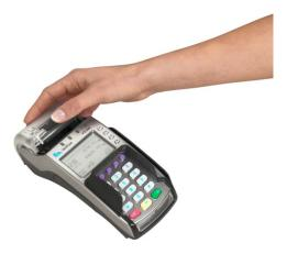
Place a printing paper roll as indicated in the picture. Make sure that a part of the paper of the roll sticks out and close the printer cover. Now tear off the protruding paper along the cut edge.
