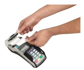
Open the cover of the printer. This is done by pulling back the printer knob and sliding the printer cover backwards. If present, remove the previous printing paper roll.
