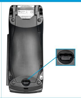
2 Use the power cable to connect the payment terminal to an outlet.
