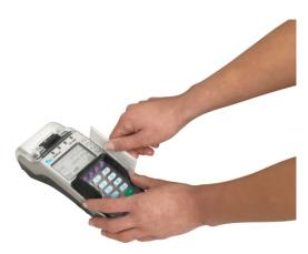
Swipe the cleaning card in a straight way and with a constant speed through the magnetic card reader of the payment terminal. The cleaning card has two cleaning strips on both sides. For the best result, swipe the card through the magnetic stripe reader twice without turning it over.
