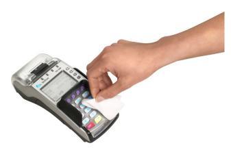
Wipe the casing, keyboard and screen of the terminal clean with a cleaning pad. Pay extra attention to the keys. Like a keyboard or telephone, for example, the keys may contain a lot of bacteria after a certain period of use.
