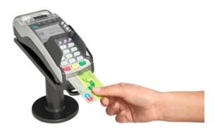
A payment card with EMV chip must be inserted into the chip card reader. The card must be inserted in the card reader with the chip facing up and toward the terminal.
