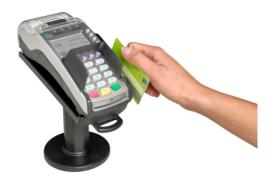
A payment card with a magnetic strip must be swiped through the magnetic card reader. The card should be swiped through the magnetic card reader with the magnetic strip facing down and toward the terminal.
