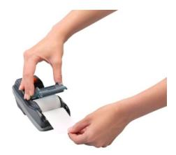
Insert the new printer roll as indicated in the above photograph. Make sure to leave a strip of paper sticking out and close the printer cover. Tear off the strip of paper along the cutting edge.
