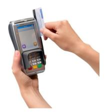
A payment card with a magnetic strip must be swiped through the magnetic card reader. The card must be swiped through the magnetic card reader with the magnetic strip facing down and towards the payment terminal.
