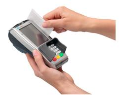
Swipe the cleaning card through the magnetic card reader of the payment terminal. Hold the cleaning card in an upright position and swipe at a constant speed. The cleaning card has two cleaning strips on both sides. The best result is obtained when you swipe the cleaning card through the magnetic card reader twice, without turning the card over.
