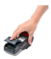
1. Press the release button and open the printer cover. Remove the old printer roll.
