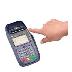
Press the release button and open the printer cover. Remove the old printer roll if necessary.
