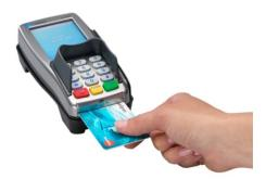
A payment card with an embedded EMV chip must be inserted in the chip card reader. The card must be inserted in the chip card reader with the chip facing up and towards the PINpad.
