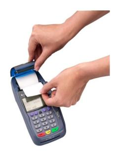
Insert the new printer roll as indicated in the above photograph. Make sure to leave a strip of paper sticking out and close the printer cover. Tear off the strip of paper along the cutting edge.
