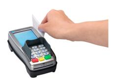
Swipe the cleaning card through the magnetic card reader. Hold the cleaning card in an upright position and swipe at a constant speed. The cleaning card has two cleaning strips on both sides. The best result is obtained when you swipe the cleaning card through the magnetic card reader twice, without turning the card over.
