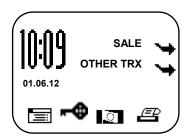
Up to eight lines can be displayed on the screen. The top line (i.e. the line above the dividing line) always states the name of the current menu.
