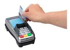
A payment card with a magnetic strip must be swiped through the magnetic card reader. The card must be swiped through the magnetic card reader with the magnetic strip facing down and towards the PINpad.
